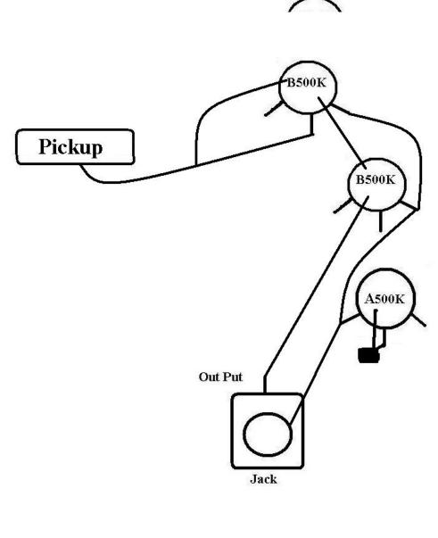
Solo MMK-10 Wiring Diagram
