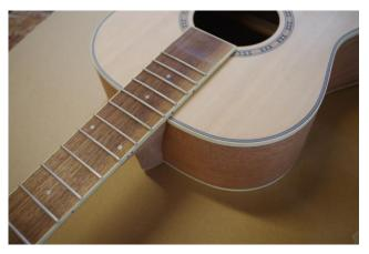
Take sandpaper and a flat sanding block (we recommend 220 or finer) and give all the surfaces on the neck and body a quick sanding to make sure you are happy with how everything feels and looks. Do not sand the fretboard (as it should still be covered in masking tape), but you could slightly sand the edges of all the binding if you find them too sharp. Slide the dovetail joint of the neck back together and make sure you are happy with all the gluing surfaces.
