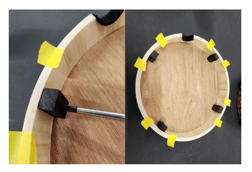
Hold the banjo inside the resonator and make sure you are nicely in the center. Mark each bracket hole, remove the banjo and drill 1/8" (4mm) %" (19mm) deep pilot holes. Using the chromed pan head screws, attach the banjo to the Resonator.
