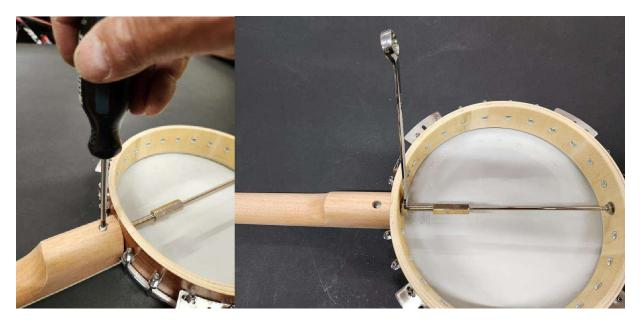
**Installing the Tail-piece:** Loosen the thumb screw on the back of the tail-piece. Remove the hex nut from the threaded rod at the bottom and insert this rod though the hole in the back strap pin. Re-install the hex nut ensuring the two hooks on the tailpiece are over the Tension Ring and tighten. (see pic)
