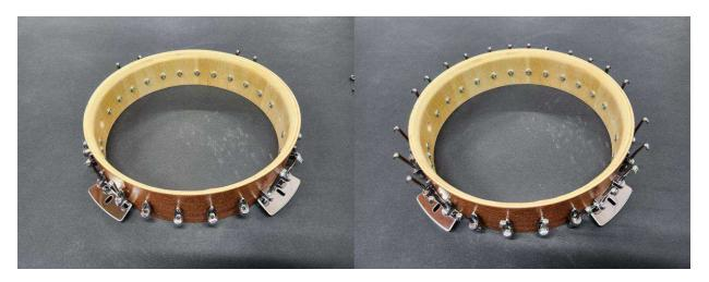
You should now have 24 evenly spaced hooks and 4 Resonator Plates evenly spaced around the Rim. Go ahead and install the strap pin in the extra hole close to the neck on the upper bout (see pic).
