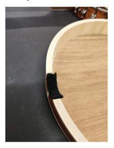
The Resonator Brackets will sit on the top edge of the Resonator. Make sure your spacing is even all the way around and mark each bracket on the rim of the Resonator.
