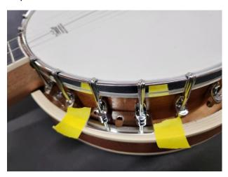
Now take the supplied block shims and install them against the inside rim of the Resonator making sure the screw is toward the back of the Resonator. Make sure you use glue before you screw these pieces in and install the screw so the top surface of the shim is even with the top rim of the Resonator. (There are 5 block shims and 5 screws supplied, but only 4 are required for this process, the fifth shim and screw are supplied in case you have a problem with one)
