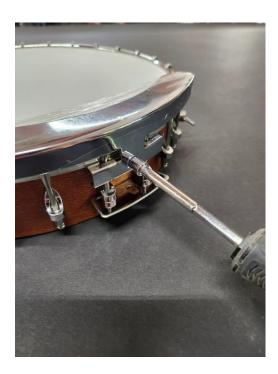
Now remove the Strap Pin from the end of the Tension Rod and one washer. Insert the opposite end through the neck hole and then re-insert the Strap Pin end and install a washer and Strap Pin on the outside of the Rim. Tighten the Strap Pin hand tight ensuring the hole is perpendicular to the top. Tighten the nut against the inside of the Rim with a small wrench. Be careful to make it tight, but not to distort the wood on the inside or outside. You are now ready to attach the neck.
